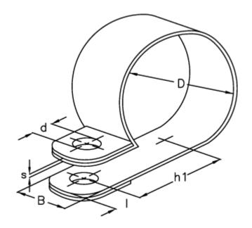
$\begin{array}{ll} d & = 10.5 \\ \text{Diameter D} = 52 \\ \text{h1} & = 40.5 \\ \text{I} & = 10.0 \\ \text{s} & = 1.0 \\ \text{Width B} & = 25 \\ \end{array}$
